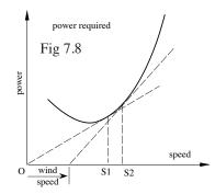
If you're interested, the exact speed required to make the best of the headwind situation is shown in Fig 7.8. The tangent from the origin, O, to the power required curve locates the minimum drag speed [S1].
